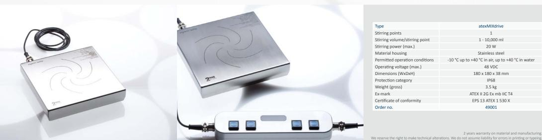
1 stirring position, 100% maintenance-free and wear-free by inductive 2mag-Magnetic-Drive concept for powerful mixing of solutions, jerk-free stirring even at low speeds.
